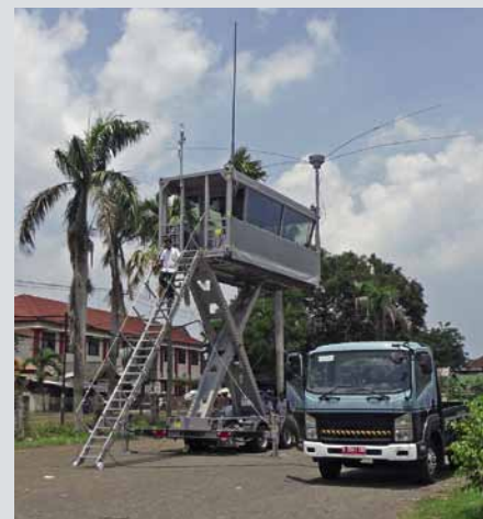
Fully equipped R&S®MX400 mobile air traffic control tower for the Indonesian ATC authority.
