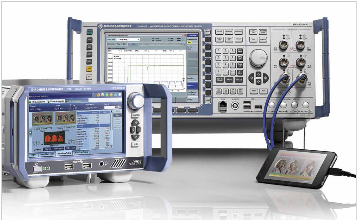
Fig. 9 Test setup with an R&S®CMW500 tester and an R&S®VTE video tester for carrying out application tests on smartphones.
