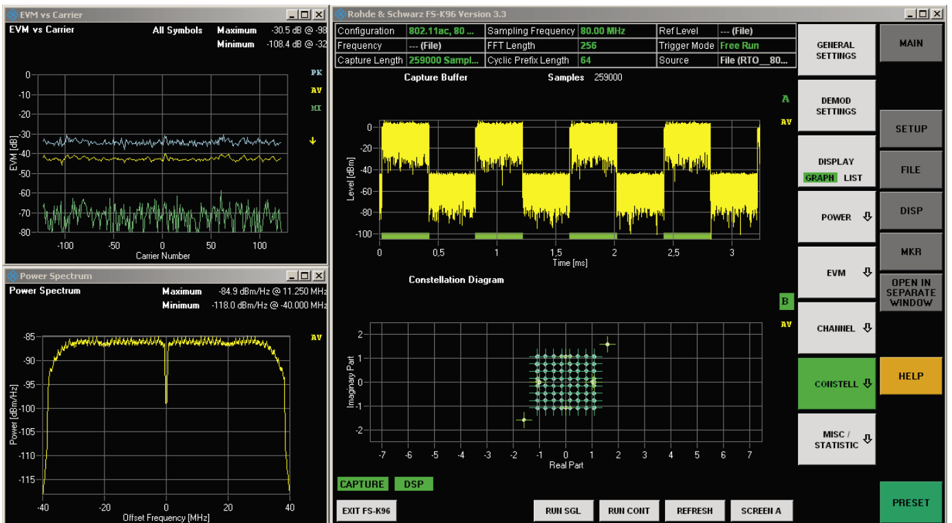
Fig. 5 The R&S®FS-K96 OFDM vector signal analysis software offers a wide range of measurements, e.g. constellation diagram or EVM over all OFDM carriers. The graphical display of results makes signal analysis easier.
